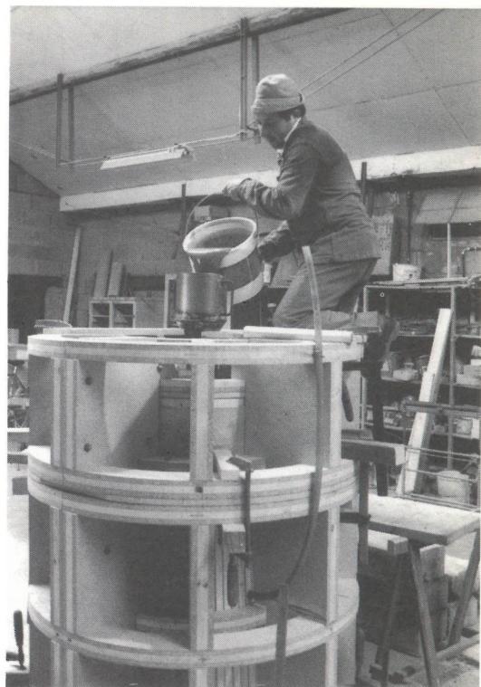
A new milestone is manufactured by "Chaux de Contern" in 1984.
